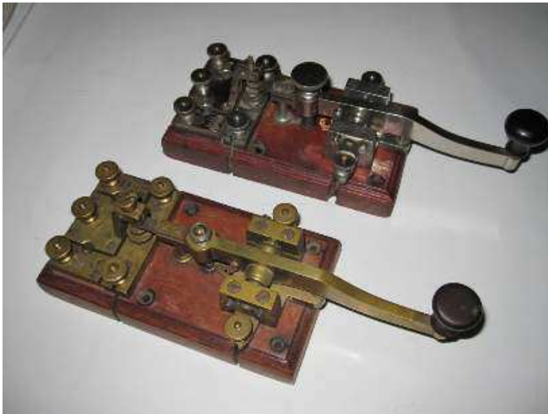
Landline telegraph keys made by the Öller factory 1857 - 1886.
